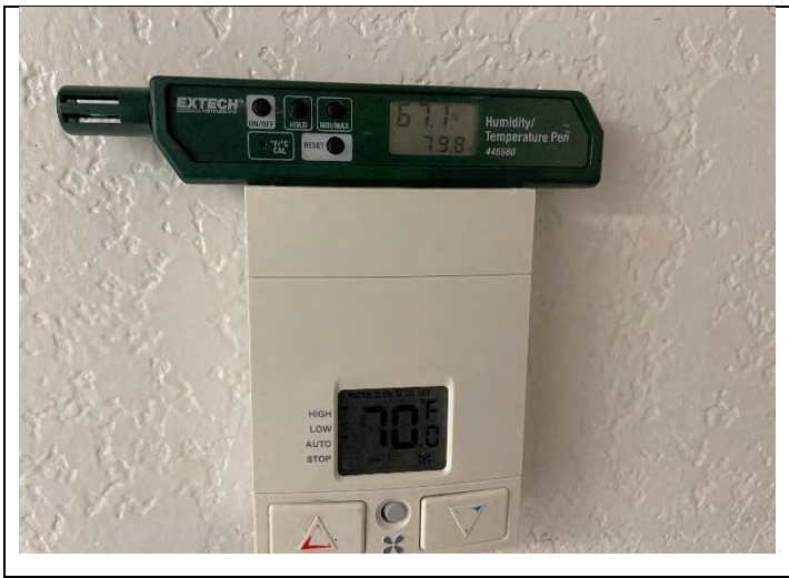
25. View of thermostat set point compared to temperature/RH pen comparison
