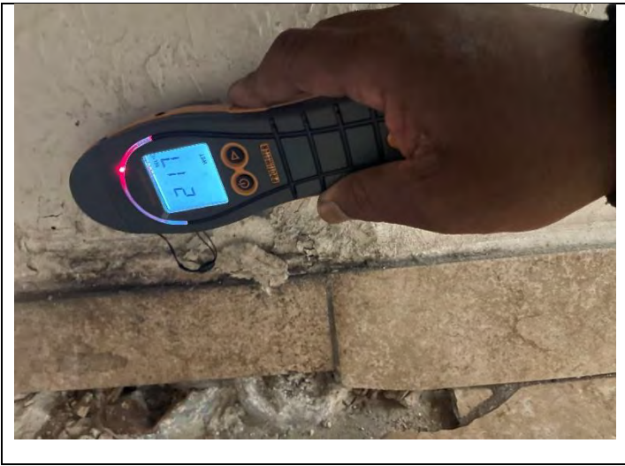
31. View of SVG and elevated moisture using Protimeter under restroom sink in PEI 307
