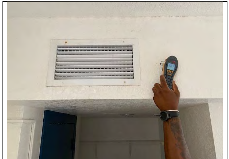
18. View of elevated moisture levels using Protimeter around supply diffuser in PEI 230
