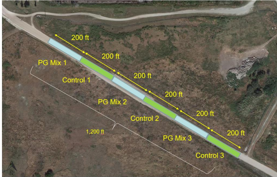
Figure 1. Aerial View of the Proposed Pilot Project Road (1200 ft) with PG-aggregate Road Bases and Respective Control Segments (200 ft each)
